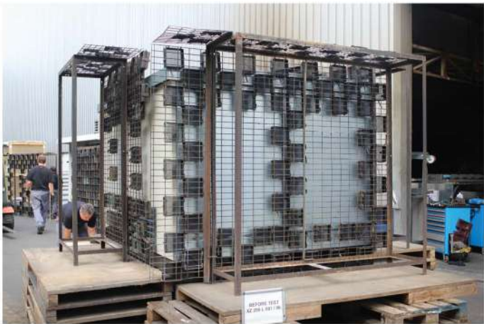
" EMP 1000-1600 PEHLA No.4 IEC 62271-202 " Before Test
