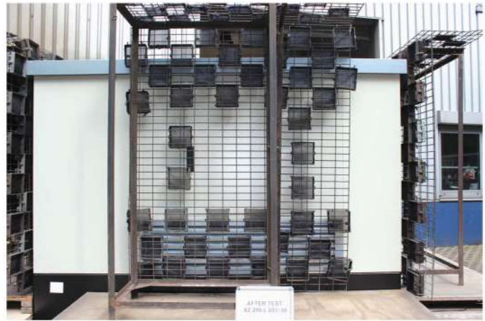
" EMP 1000-1600 PEHLA No.4 IEC 62271-202 " After Test
